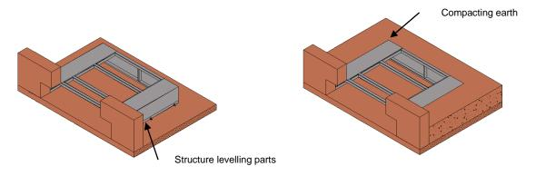
Then place the leveller on the framework, fitting it into the front wall. Once in place, it will be anchored to the permanent framework with weld spots.
