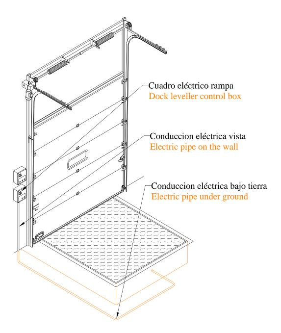
Once everything is secured, pass the cables through and connect, pursuant to the attached electrical diagram which is inside the electrical control panel. (See electrical control panel connections, page 19)
