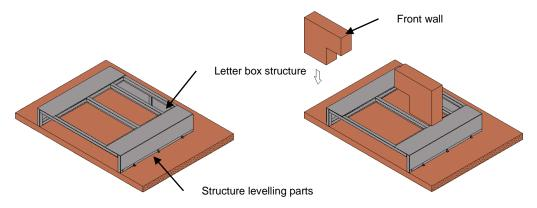
Once the permanent framework has been anchored and levelled and the front wall built, the earth will be supplied for compacting. Compacting of earth will ONLY be done up to the level of the letter box structure.
