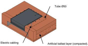
Open all the claws and weld the ends of the claws of the leveller to the framework of the building floor and add the final paving concrete.
