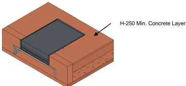
Lastly, after the paving has hardened and been ground and finished, remove the protective cover.
