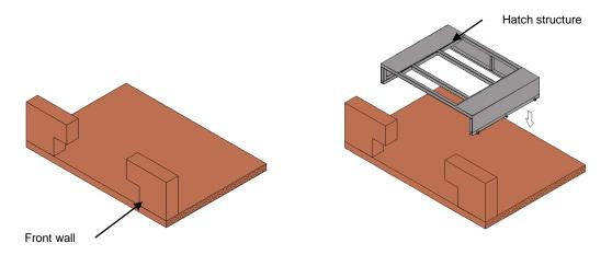
Once the permanent framework is anchored, fill with earth and compact it. Compacting of earth will ONLY be done up to the level of the letter box structure.
