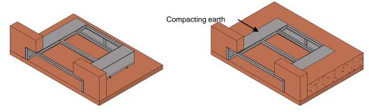
Then place the leveller on the framework, fitting it into the front wall. Once in place, it will be anchored to the permanent framework with weld spots.
