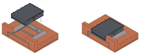
Install the  $\emptyset$ 50 tube for the electrical ducts. Install a cable guide in the tube or pass the cables directly from the leveller through the tube.
