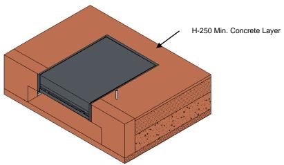
Lastly, after the paving has hardened and been ground and finished, remove the protective cover.
